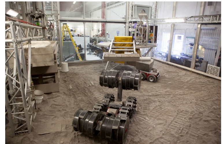
NASA RASSOR excavator testing at KSC in BP-1 lunar simulant
